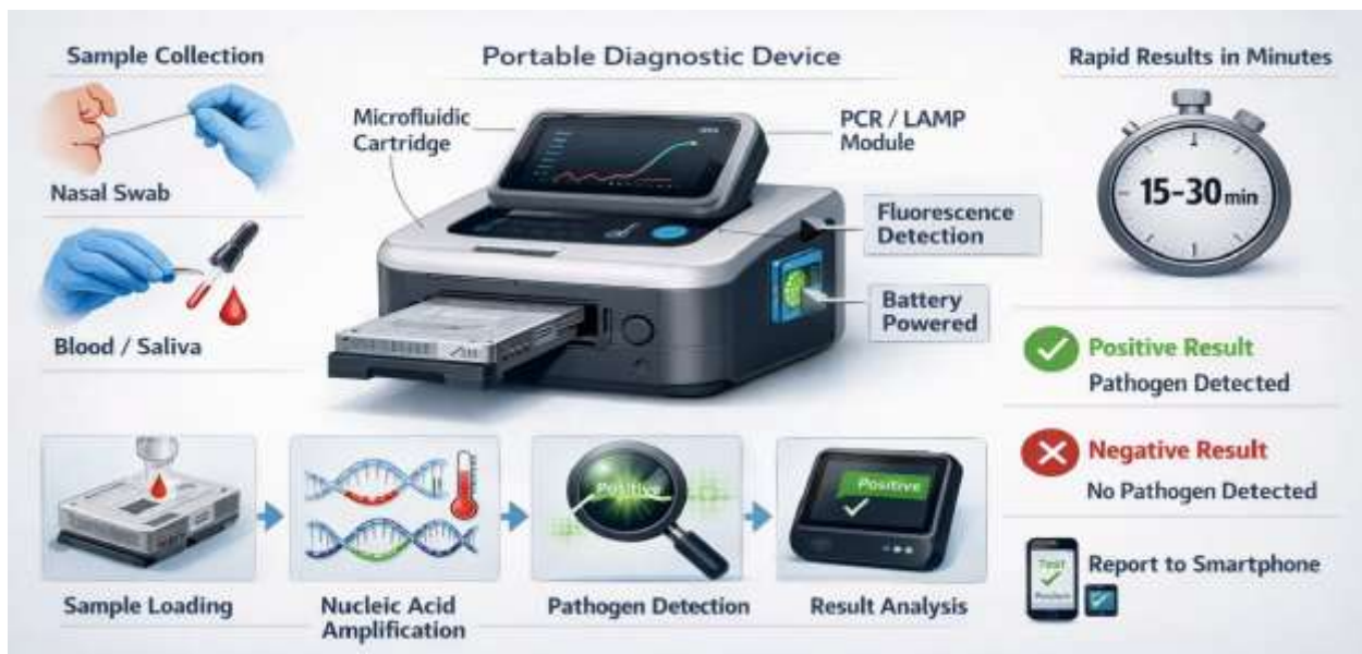
Figure 4.3 Point-of-Care Molecular Diagnostic Device for Rapid Pathogen Detection.
